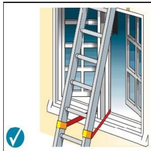
Ladder tied at the top stiles (correct for access) Tying part way down working on, but not for access)
