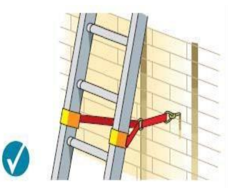
near the base Securing at the base
